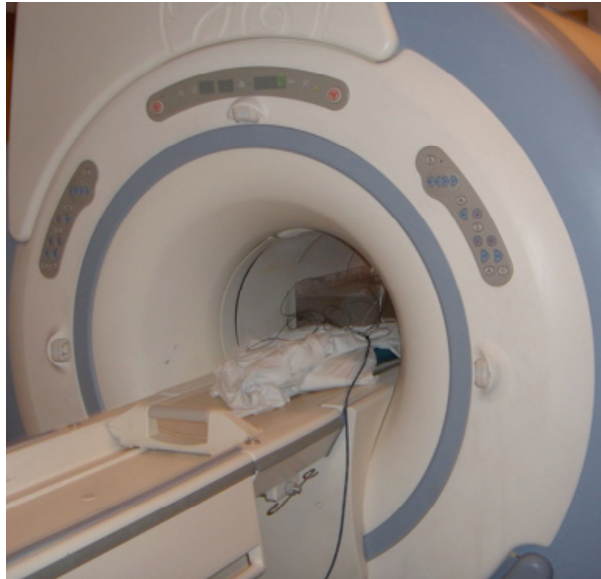
FIGURE 6. Experimental set up showing the 3-Tesla MR system and head/torso phantom used for the evaluation of MRI-related heating for the On-X Prosthetic Heart Valve, Conform-X Mitral Heart Valve Prosthesis; Size 25-33. Note the cables going to the fluoro optic thermometry probes of the Luxtron Thermometry System.
