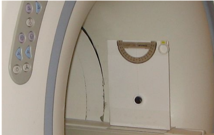
FIGURE 3. The deflection angle test conducted at 3-Tesla on the On-X Prosthetic Heart Valve, Conform-X Mitral Heart Valve Prosthesis; Size 25-33. Note the deflection angle of 1-degree measured in the 3-Tesla MR system.
